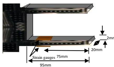
Fig. 1. The gripper with strain gauge mounted
