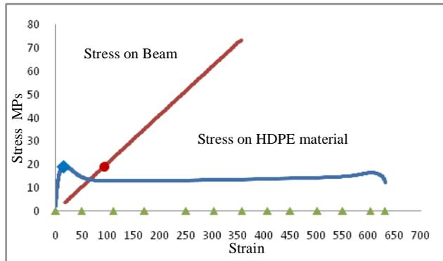
Fig. 7. Stress/Strain of the beam (gripper) and the gripped object HDPE materials
