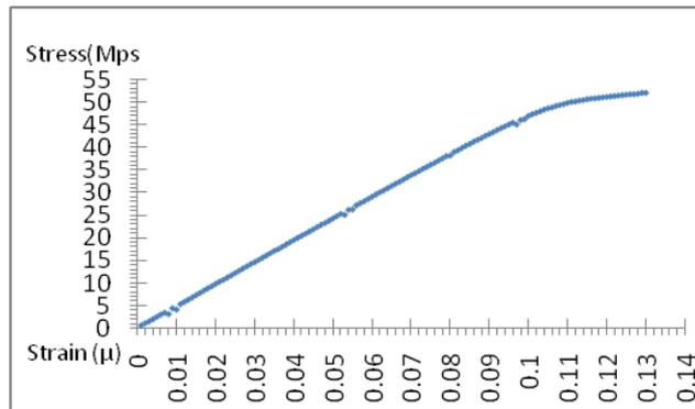
Fig. 5. Stress-Strain curve for a typical grade of Phenol-Formaldehyde (Bakelite)
