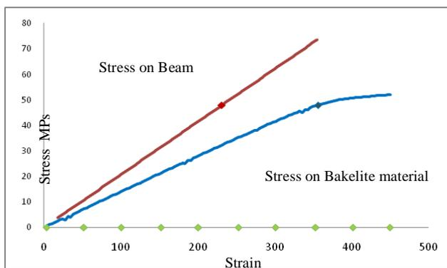
Fig. 8. Stress/Strain of the beam (gripper) and the gripped object (Bakelite).
