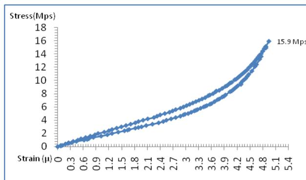
Fig. 6. Stress-strain curve for a typical grade of natural rubber
