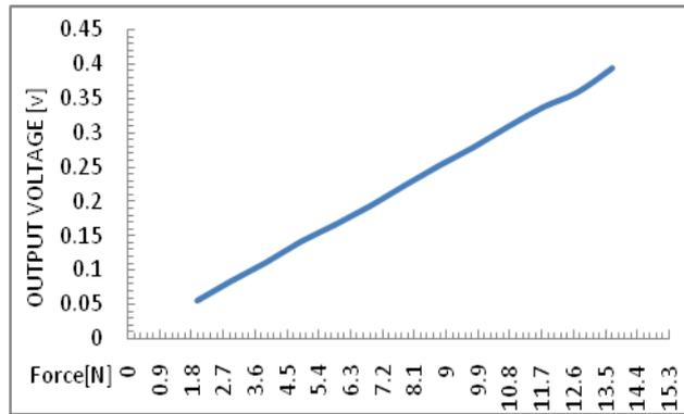
Fig. 3. Calibration results for output voltage using applied force
