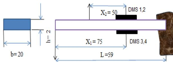
Fig. 2. Dimensions of the gripping rod
