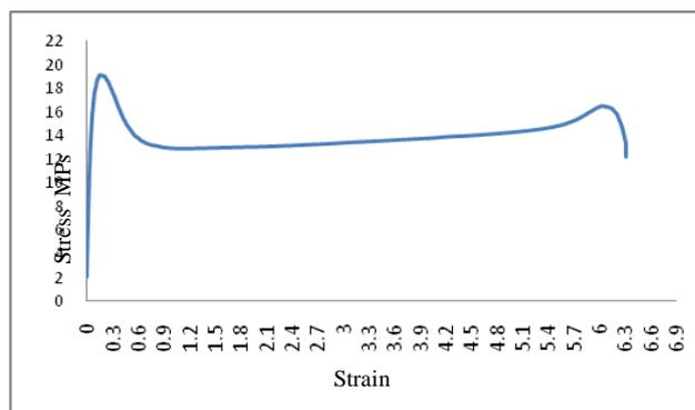
Fig. 4. Stress-strain curve for a typical grade of HDPE
