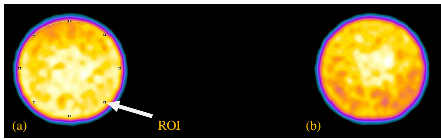
Fig. 3 (a) and (b) Transverse images of a uniform region of the phantom (a) without and (b) with material filter
